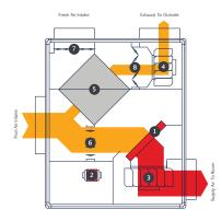
The XF uses controlled fan nowe and the ability to re-circulate the pool room air to reduce ventilation to a minimum, saving unnecessary heat loss and electrical energy.
