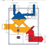
The XF automatically provides dilution with fresh air to maintain air quality.
