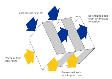
A recuperator is a 'passive' device that has no moving mechanical parts and consumes no power in order to function. It relies upon air being passed through it by operation of the fan systems.
